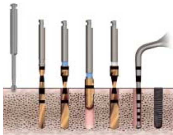
Guide Drill Twist Drill 2.0 Twist Drill 2.7 Cortical Drill 2.7/3.0 Twist Drill 2.85 OsseoSpeed™ TX 3.0 S 13 mm
